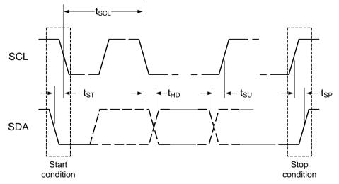
Figure 2: I<sup>2</sup>C Data Transfer
