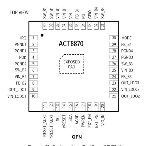
Figure 1: Pin Configuration – Top View – QFN55-40
