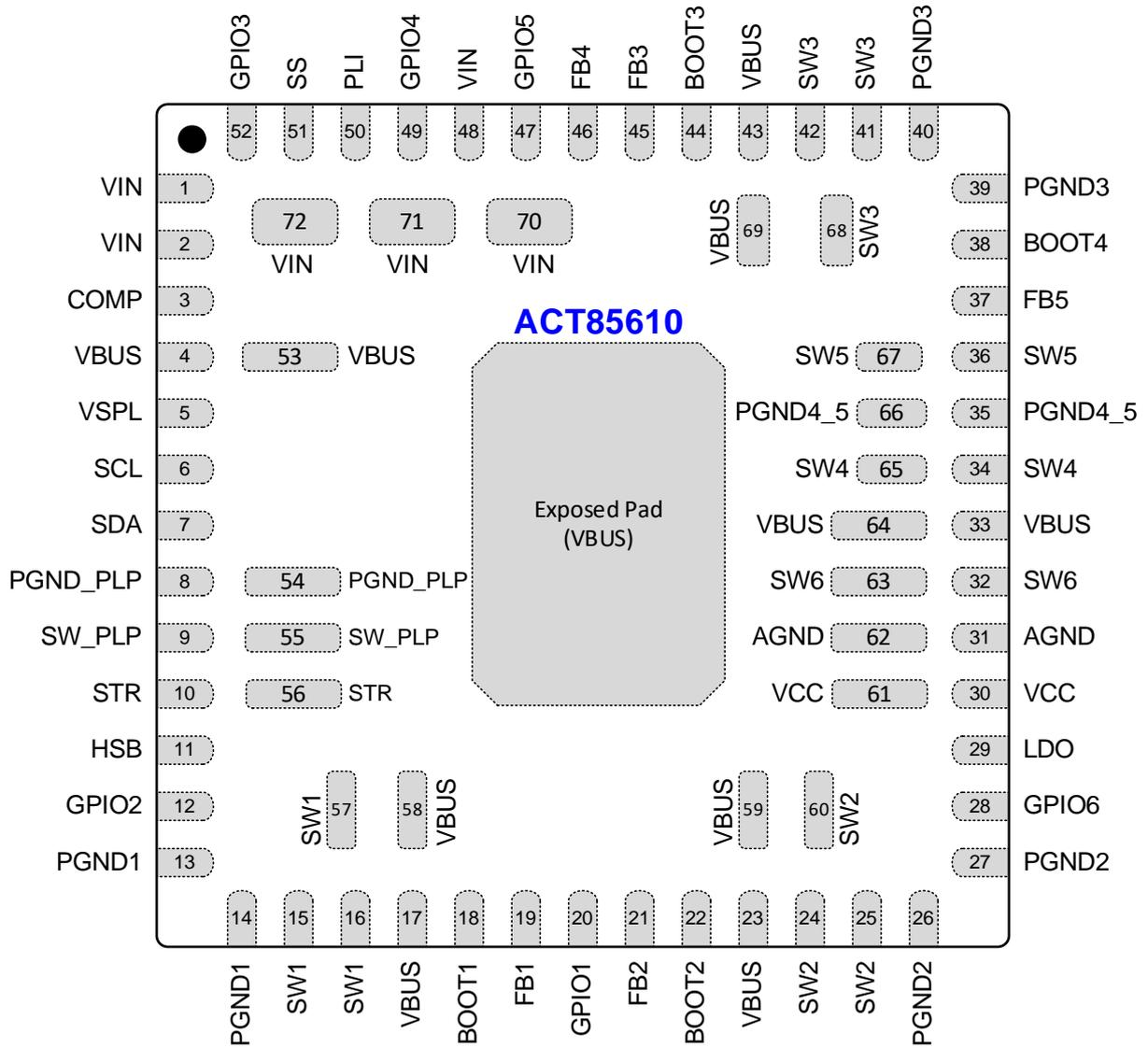
Figure 3: Pin Configuration – Top View – QFN6x6-52
