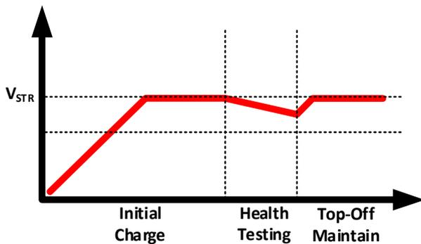
Figure 7: Storage Voltage at Different Stages
