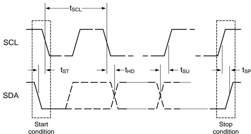
**Figure 4: I<sup>2</sup>C Data Transfer**
