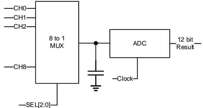
Figure 9: ADC Block Diagram
