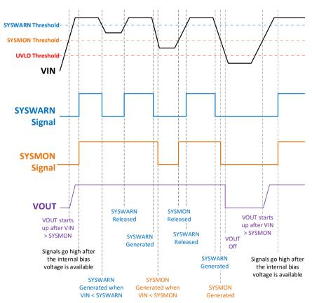
Figure 5: SYSMON and SYSWARN Signals
