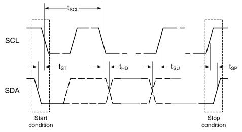
Figure 2: I<sup>2</sup>C Data Transfer
