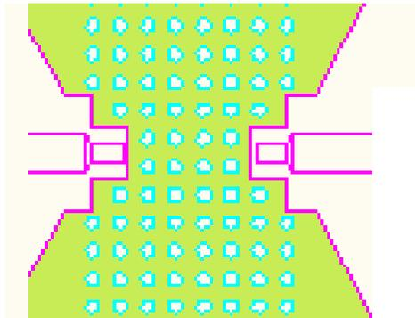
The pad pattern shown above has been developed and tested for optimized assembly at Qorvo. The PCB land pattern has been developed to accommodate lead and package tolerances. Since surface mount processes vary from company to company, careful process development is recommended.
