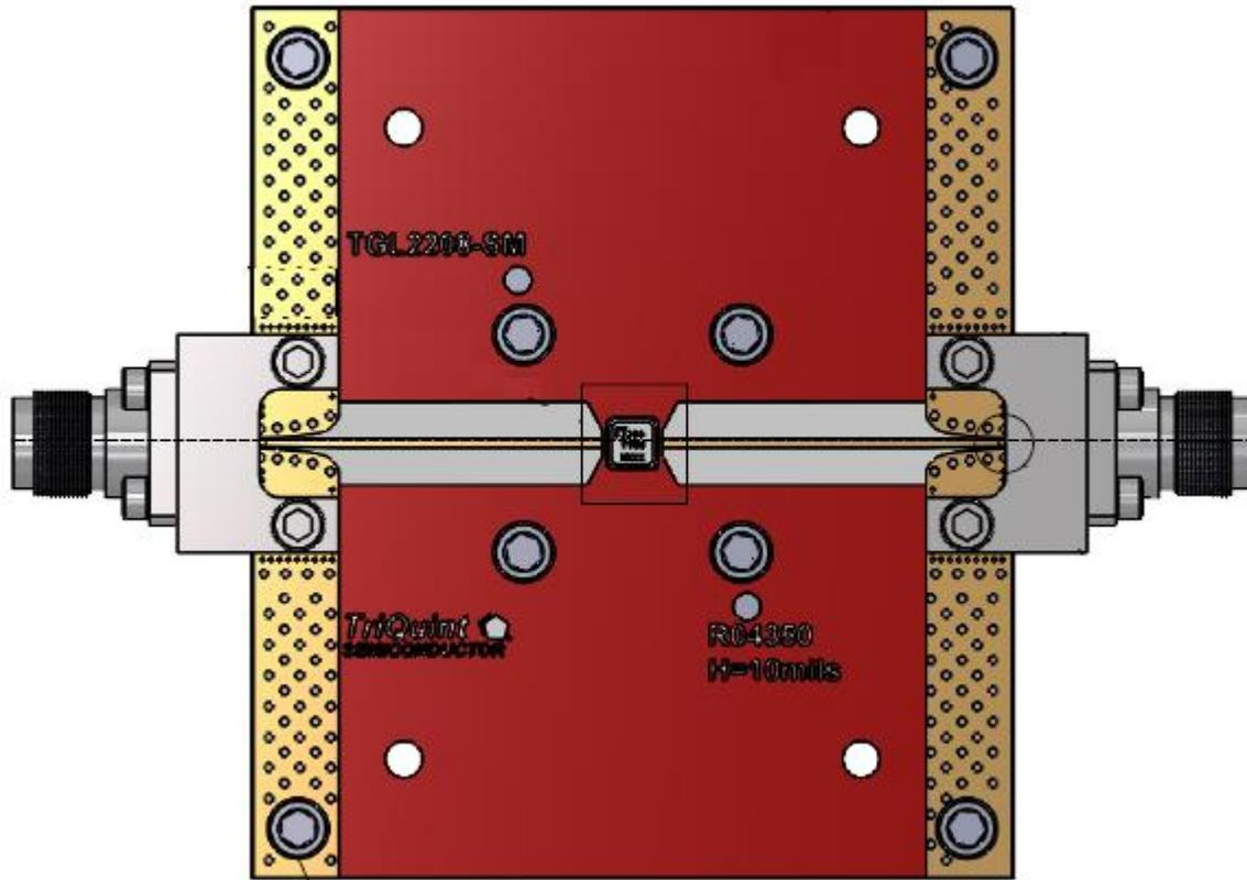
RF layer is 0.010" thick Rogers RO4350. Metal layers are 0.5-oz copper. Microstrip 50  $\Omega$  line width is 0.021". The microstrip line taper at the connector interface is optimized for the Southwest Microwave end-launch connector 1092-01A-5.
