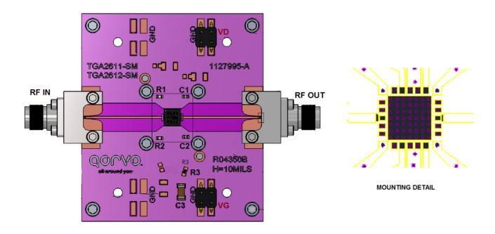
The microstrip line at the connector interface is optimized for the Southwest Microwave end launch connector 1092-01A-5.
