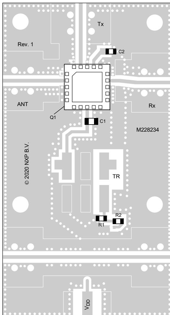
Figure 3. AFRX5G372 Application Circuit Component Layout
