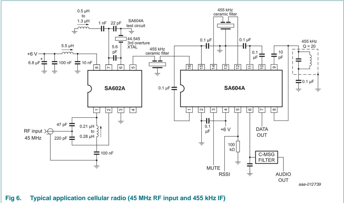
Fig 6. Typical application cellular radio (45 MHz RF input and 455 kHz IF)
