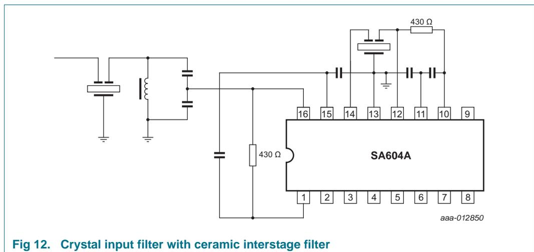
Fig 12. Crystal input filter with ceramic interstage filter
