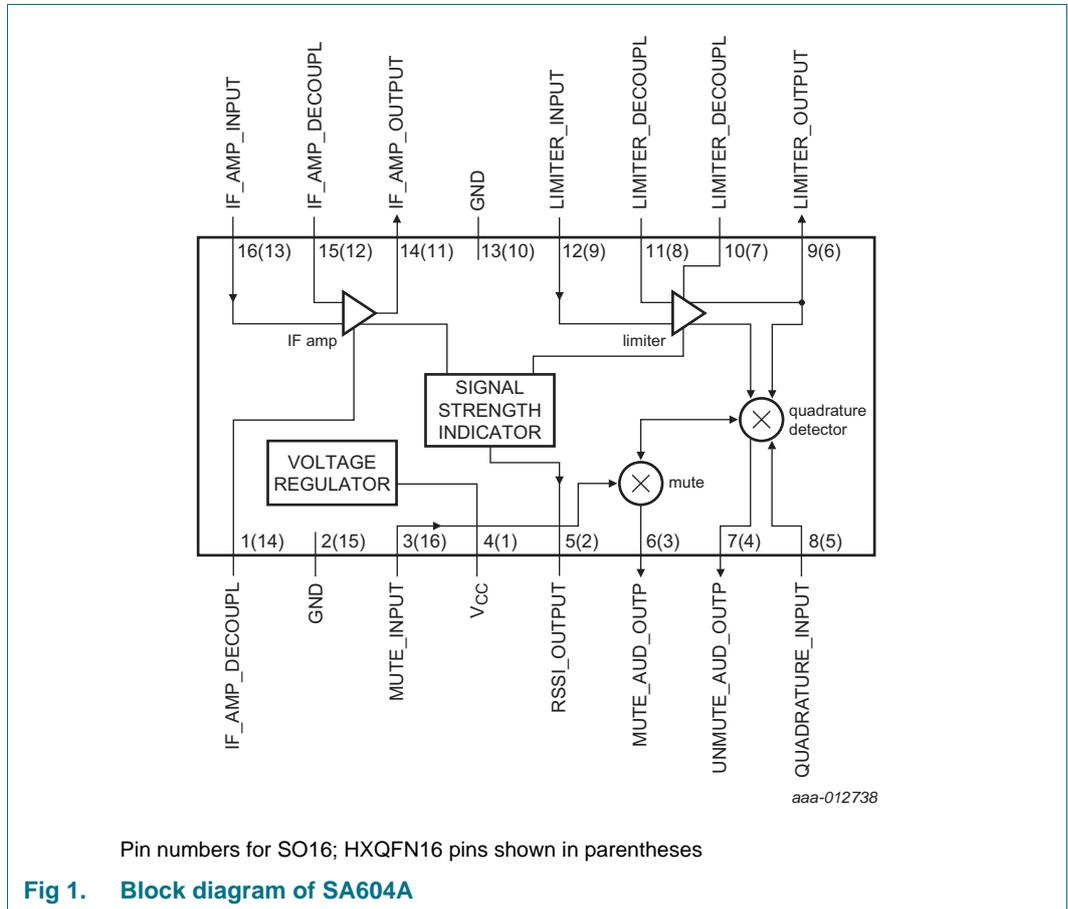
Fig 1. Block diagram of SA604A
