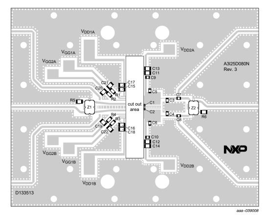
Figure 4. A3I25D080N Test Circuit Component Layout — 2300-2400 MHz
