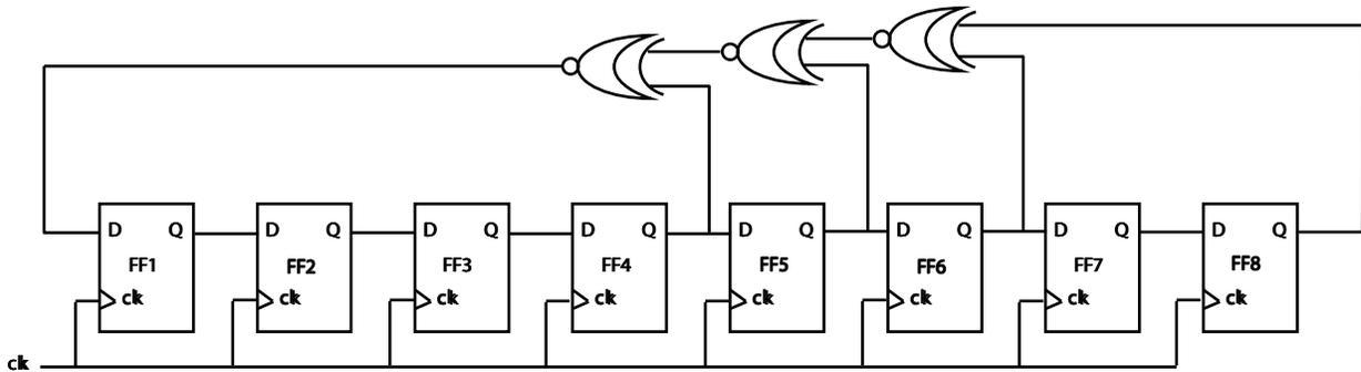
Figure 14. Diagram of linear feedback shift register (LFSR)
