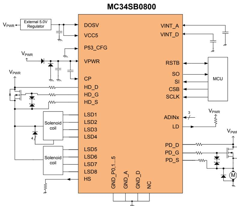
Figure 1. SB0800 simplified 5.0 V application diagram
