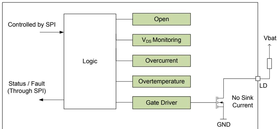
Figure 10. Low-side driver for resistive load diagram block
