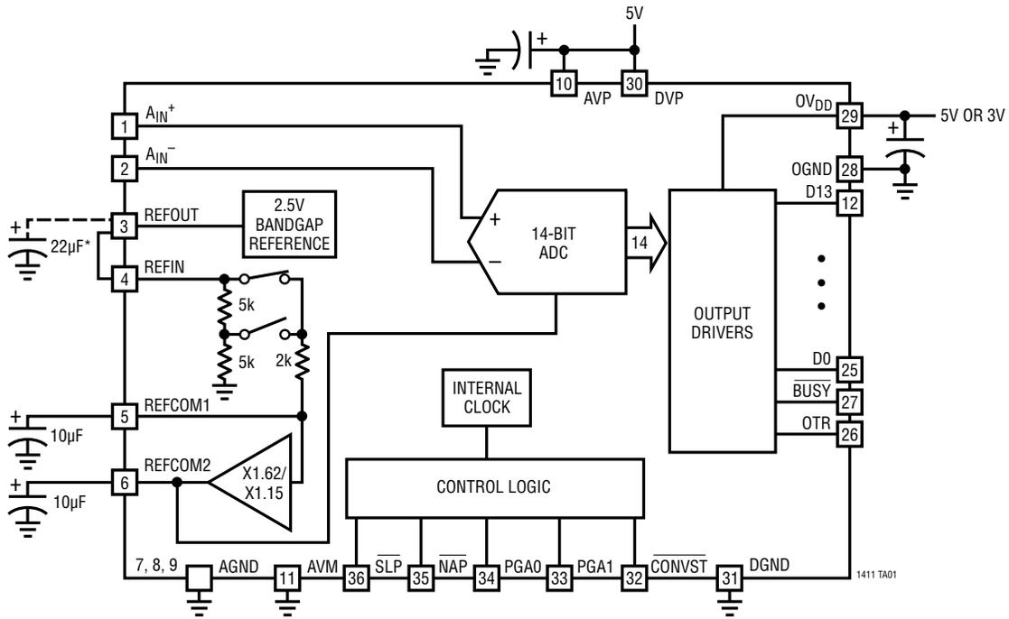
\*A 22µF CAPACITOR IS NEEDED IF REFOUT IS USED TO DRIVE AIN-
