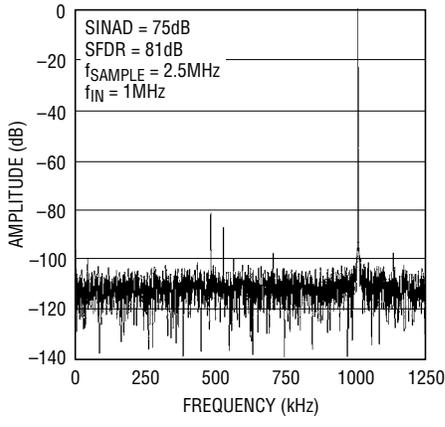
**Figure 2b. LTC1411 4096 Point FFT, Input Frequency = 1MHz**
