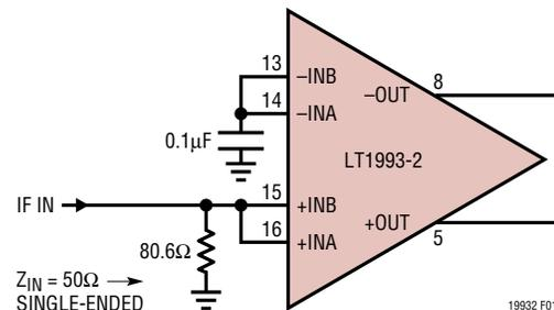
**Figure 1. Input Termination for Single-Ended  $50\Omega$  Input Impedance**
