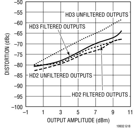
**Distortion (Filtered) vs Frequency
