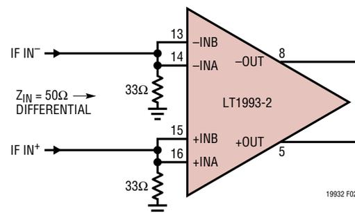
**Figure 2. Input Termination for Differential  $50\Omega$  Input Impedance**
