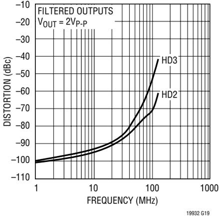
**Distortion (Filtered) vs Frequency
