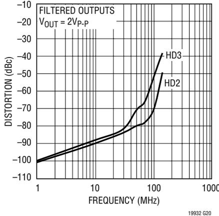
**Distortion (Filtered) vs Frequency
