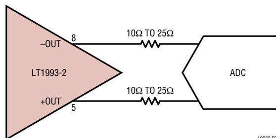
**Figure 5. Adding Small Series R at LT1993-2 Output**
