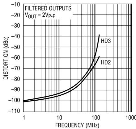
**Distortion (Filtered) vs Frequency Differential Input,  $R_{LOAD} = 100\Omega$**
