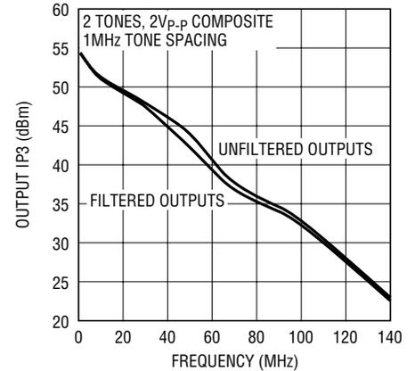
**Distortion (Filtered) vs Frequency Differential Input, No  $R_{LOAD}$**
