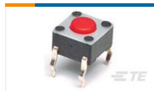
TE 产品编号1-1825910-0 FSM6JH=6MM TACT SWITCH, HIGH TEMP
