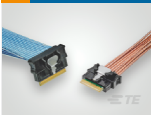
TE 产品编号2821750-2 SLIVER C/A, 50P, STR TO STR,25GHZ, 100OHM
