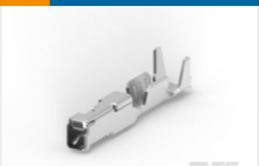
TE 产品编号2098762-8 Contact,female0.64, 22 AWG, CuNiSi, Sn
