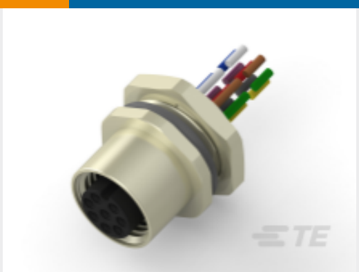
TE 产品编号T4171320008-001 M12,FRONT MOUNT,FEMALE, A, 8P, 0.2M WIRE
