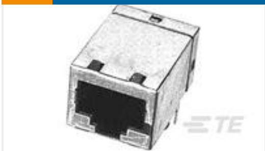
TE 产品编号1-1734264-1 M/J,RJ45,Side entry,8P8C,R/A,1
