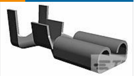
TE 产品编号42452-2 FASTON 187 TERMINAL REC 20-16 AWG TPBR
