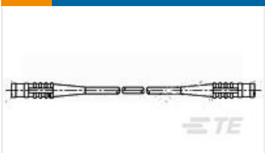
TE 产品编号1337814-1 50 OHM COAX SMB STR PLUG STR P
