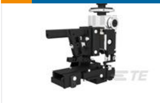
TE 产品编号2151115-1 OCEAN_2.0_Applicator-S-062F110F
