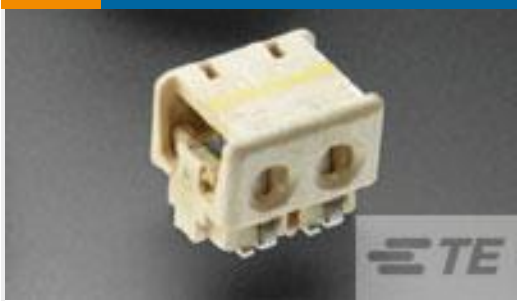
TE 产品编号1-2106003-2 Connector, SMT-IDC, 2 POS, 20 AWG
