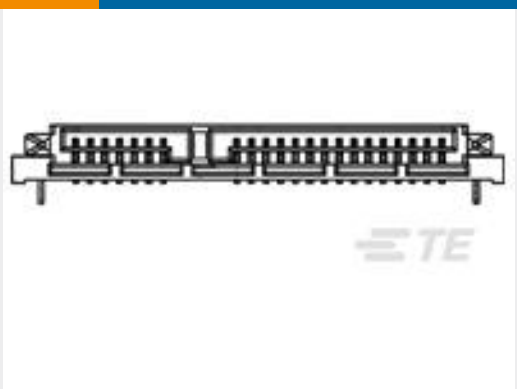
TE 产品编号2023246-2 ASS'Y SATA REC. R/A SMT TYPE 3.45H
