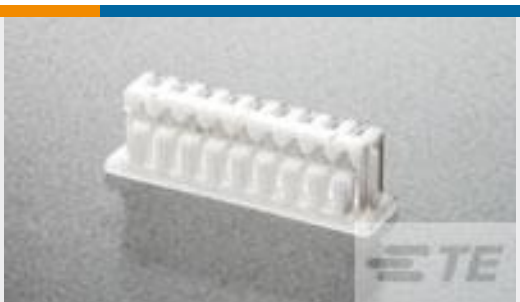
TE 产品编号1-440146-0 1.25mm WTB Socket, Housing, 10p
