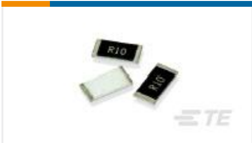
TE 产品编号1-2176051-2 RLP73N 1J R15 1% 1K RL
