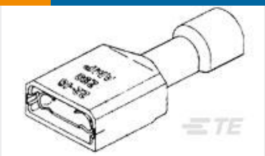
TE 产品编号3-350819-2 ULTRA-FAST 250 ASY REC 16-14 AWG TPBR
