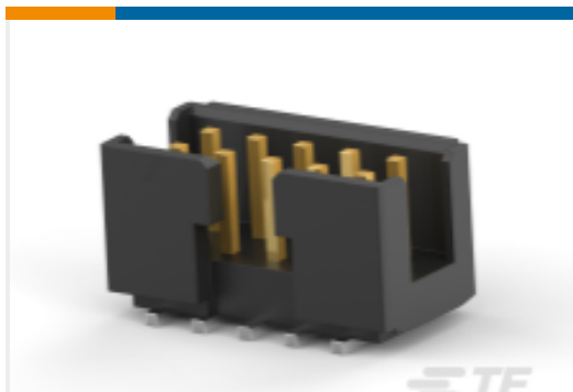
TE 产品编号1-2373376-0 10P,2MM,SHRD HDR,DRV,T,SMD,0.1 AU,TB
