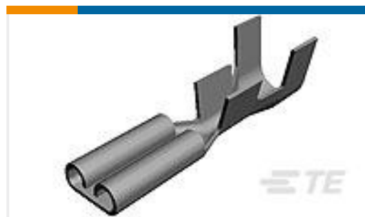
TE 产品编号170048-2 110 FASTON, REC., 24-20 AWG, TPBR
