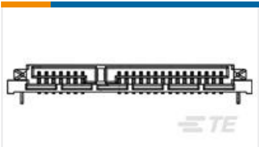
TE 产品编号2023246-2 ASS'Y SATA REC. R/A SMT TYPE 3.45H
