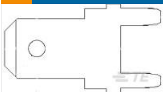
TE 产品编号1217057-1 187 FASTON,PCB TAB,TPBR
