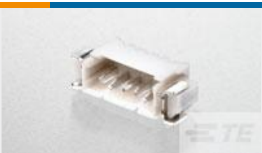
TE 产品编号1-1734261-2 1.25 WTB, HDR, SMT, RA, 12P
