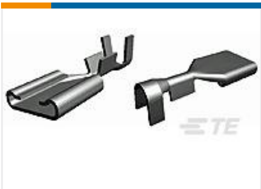
TE 产品编号61202-1 FASTON 250 RECEPTACLE 26-22 AWG BR
