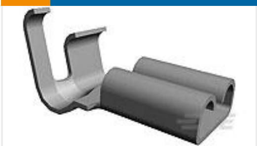
TE 产品编号1742370-2 187 FASTON, FLAG, REC., 18-14 AWG, TPBR
