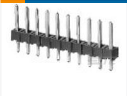
TE 产品编号146274-8 08 MODII HDR SRST B/A .100CL
