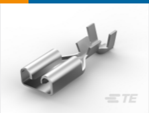
TE 产品编号2232974-1 187 FASTON,REC.,24-20 AWG,BR
