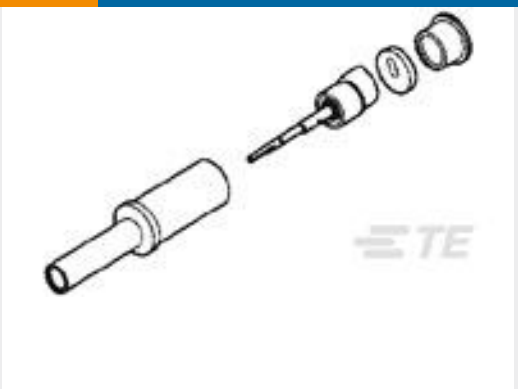
TE 产品编号1757624-1 SZ 8 COAX PIN,RG142,HEX CRIMP
