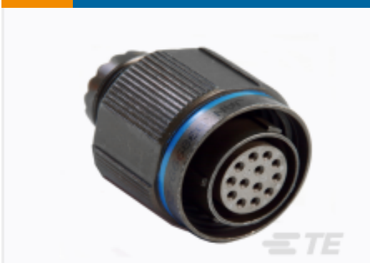
TE 产品编号YDTS26F11-05BAV001 Straight Plug: D38999, 11-05 Insert, Electroless Nickel Plating
