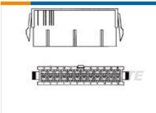
TE 产品编号2-794953-0 20P PM PLUG VAL-U-LOK V2
