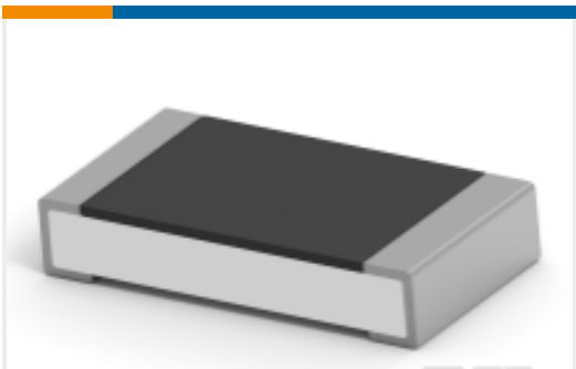
TE 产品编号2176390-3 RQ 1206 1K21 0.1% 10PPM 5K RL
