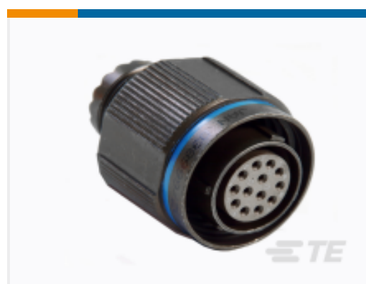
TE 产品编号 CAT-D38999-DTS19G Straight Plug: D38999, 21-39 Insert, Electroless Nickel Plating
