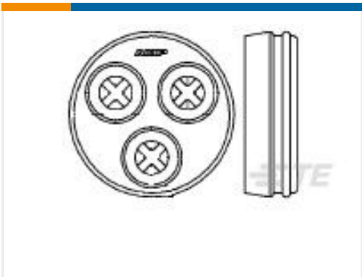
TE 产品编号213899-1 CPC SEAL ASSY KIT, SRS 5, 17-3
