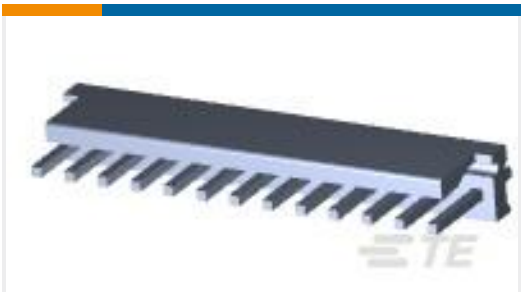
TE 产品编号1-640445-3 13P MTA156 HDR Assy FL/STR SN
