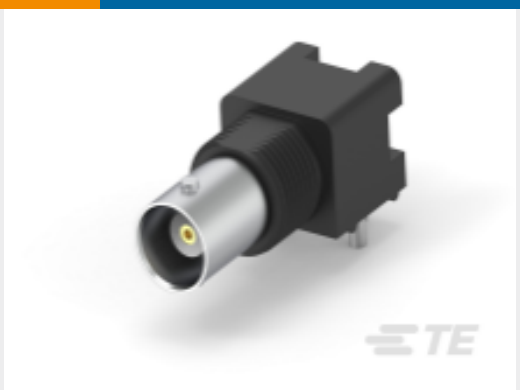
TE 产品编号226990-1 BNC Right Angle M Jack RF Connector, 50 Ohm, Bayonet Coupling Mechanism
