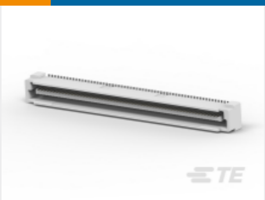
TE 产品编号1-5177986-5 Free Height Plug Connector: Board-Board, Vertical, 120, 0.8mm
