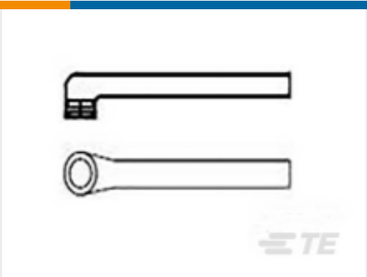
TE 产品编号462378-000 Low Profile Heat Shrink Boots: Poly Mold, Lipped, Right Angle
