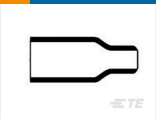
TE 产品编号808511-000 Heat Shrink Boots: Non Lipped, Straight
