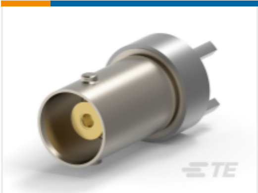
TE 产品编号414460-1 BNC Vertical Male (Jack) RF Connector, 50 Ohm, Bayonet Coupling Mechanism
