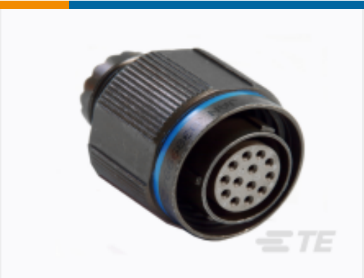
TE 产品编号YDTS26F15-05SNV001 Straight Plug: D38999, 15-05 Insert, Electroless Nickel Plating
