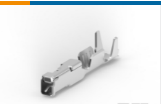
TE 产品编号2098762-3 Contact,female 0.64, 26 AWG, CuNiSi, Sn
