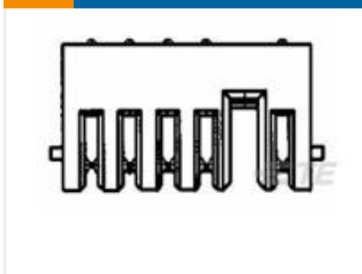
TE 产品编号1473971-2 REC ASS'Y V TYPE FOR 2.5MM PIT
