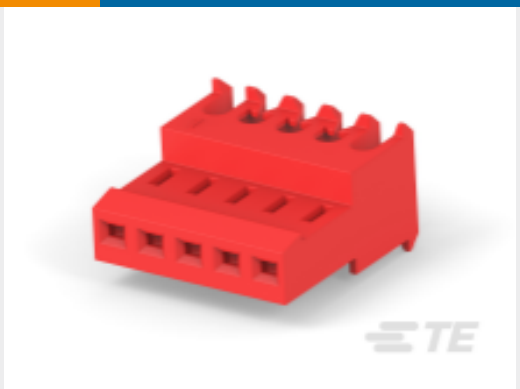
TE 产品编号3-641190-9 Nylon Gold Plated Receptacle: 2.54 mm, No Mating Alignment, MTA 100
