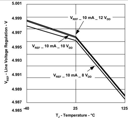
Figure 8. Line Voltage Regulation (I<sub>LOAD</sub> = 10 mA) vs Temperature
