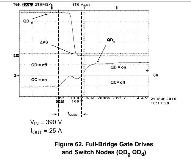
Figure 62. Full-Bridge Gate Drives and Switch Nodes (QD<sub>g</sub> QD<sub>d</sub>)
