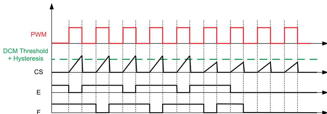
**Figure 41. Moving from CCM to DCM Mode**
