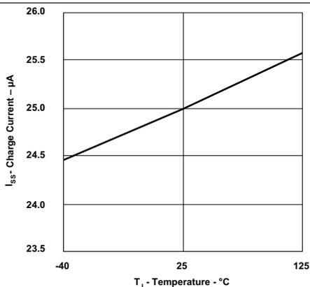
Figure 15. I<sub>SS</sub> Charge Current vs Temperature
