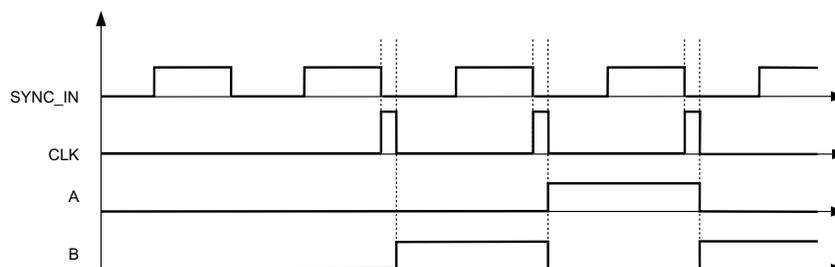
Figure 44. SYNC\_IN (Slave Mode) Timing Diagram
