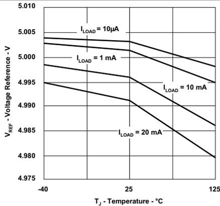
Figure 7. Voltage Reference (VDD = 12 V) vs Temperature
