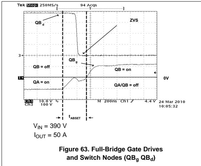
Figure 63. Full-Bridge Gate Drives and Switch Nodes (QB<sub>g</sub> QB<sub>d</sub>)
