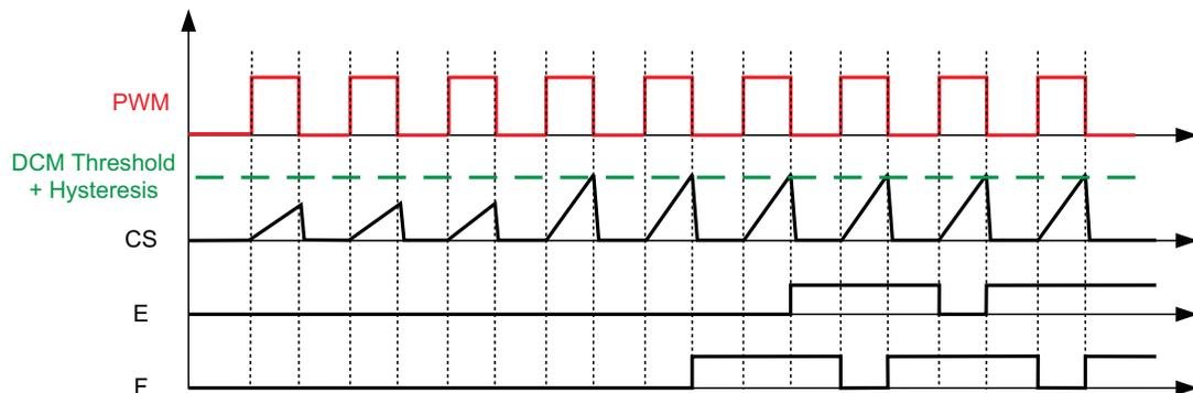
**Figure 40. Moving from DCM to CCM Mode**
