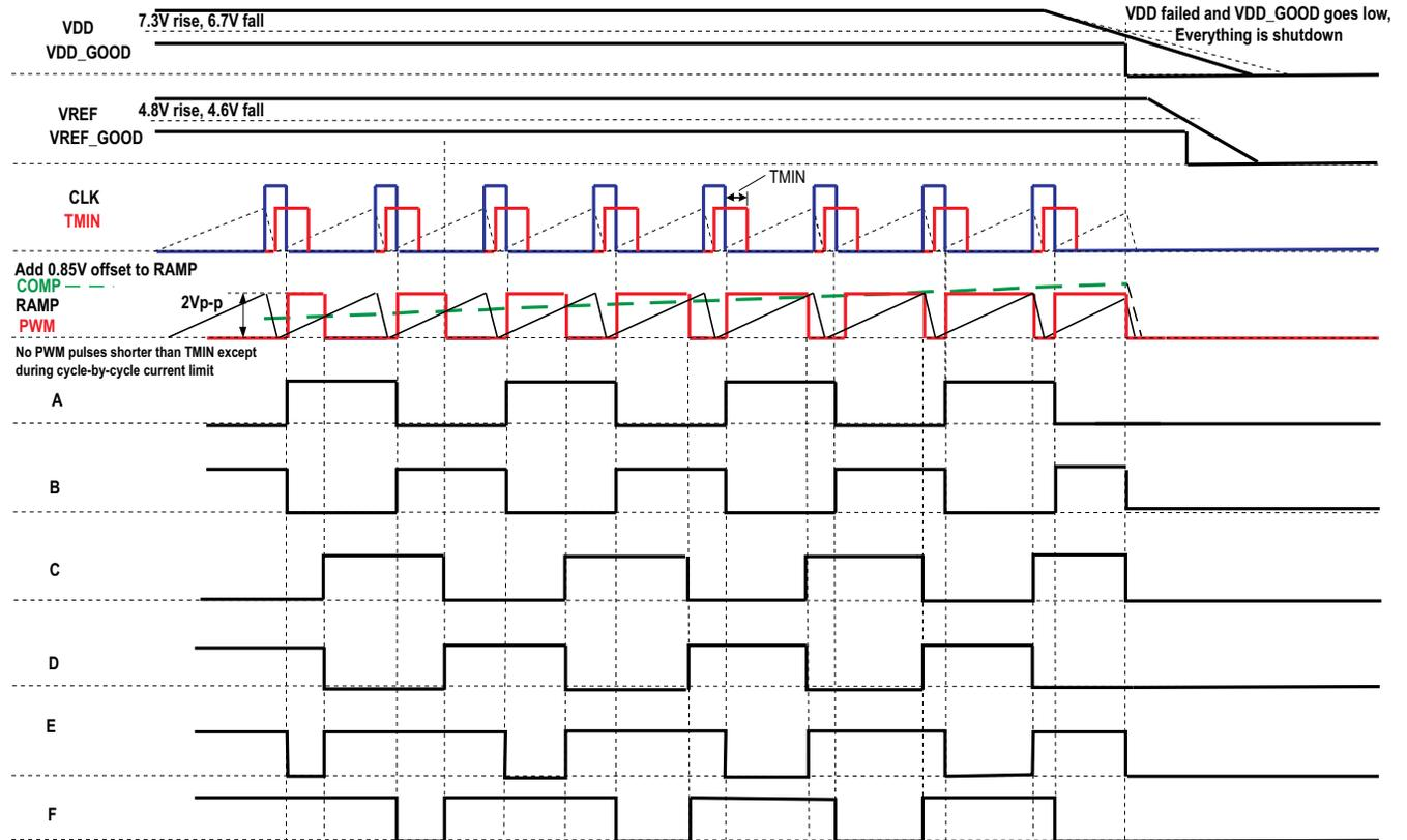
No output delay shown, COMP-to-RAMP offset not included.
