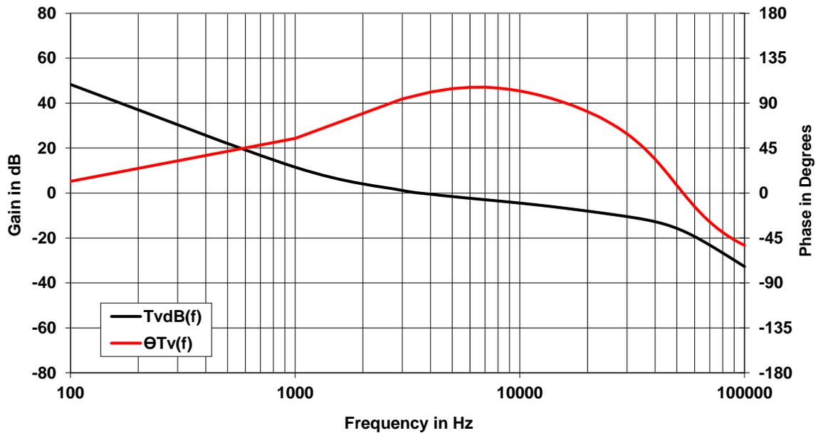
**Figure 51. Loop Gain and Phase vs Frequency**
