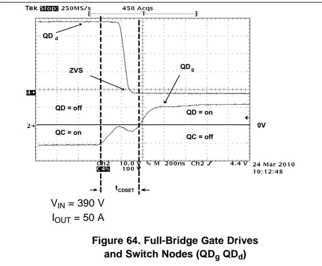
Figure 64. Full-Bridge Gate Drives and Switch Nodes (QD<sub>g</sub> QD<sub>d</sub>)
