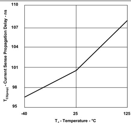
Figure 20. Current Sense Propagation Delay vs Temperature
