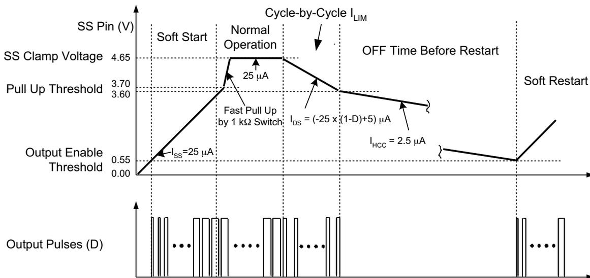
Figure 42. Timing Diagram of Soft-Start Voltage  $V_{SS}$
