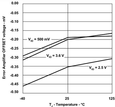
Figure 13. Error Amplifier Offset Voltage vs Temperature
