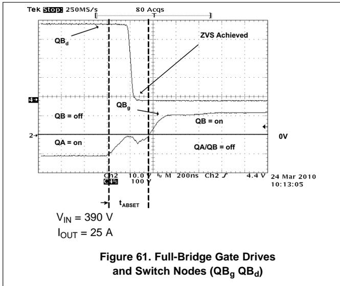
Figure 61. Full-Bridge Gate Drives and Switch Nodes (QB<sub>g</sub> QB<sub>d</sub>)
