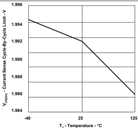
Figure 19. Current Sense Cycle-by-Cycle Limit vs Temperature
